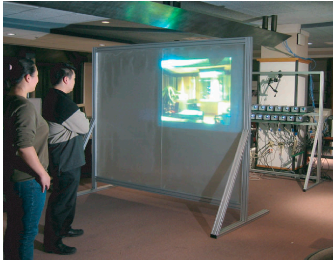
Fig. 2. Multi-point of view stereoscopic projection system with a lenticular lens screen.
